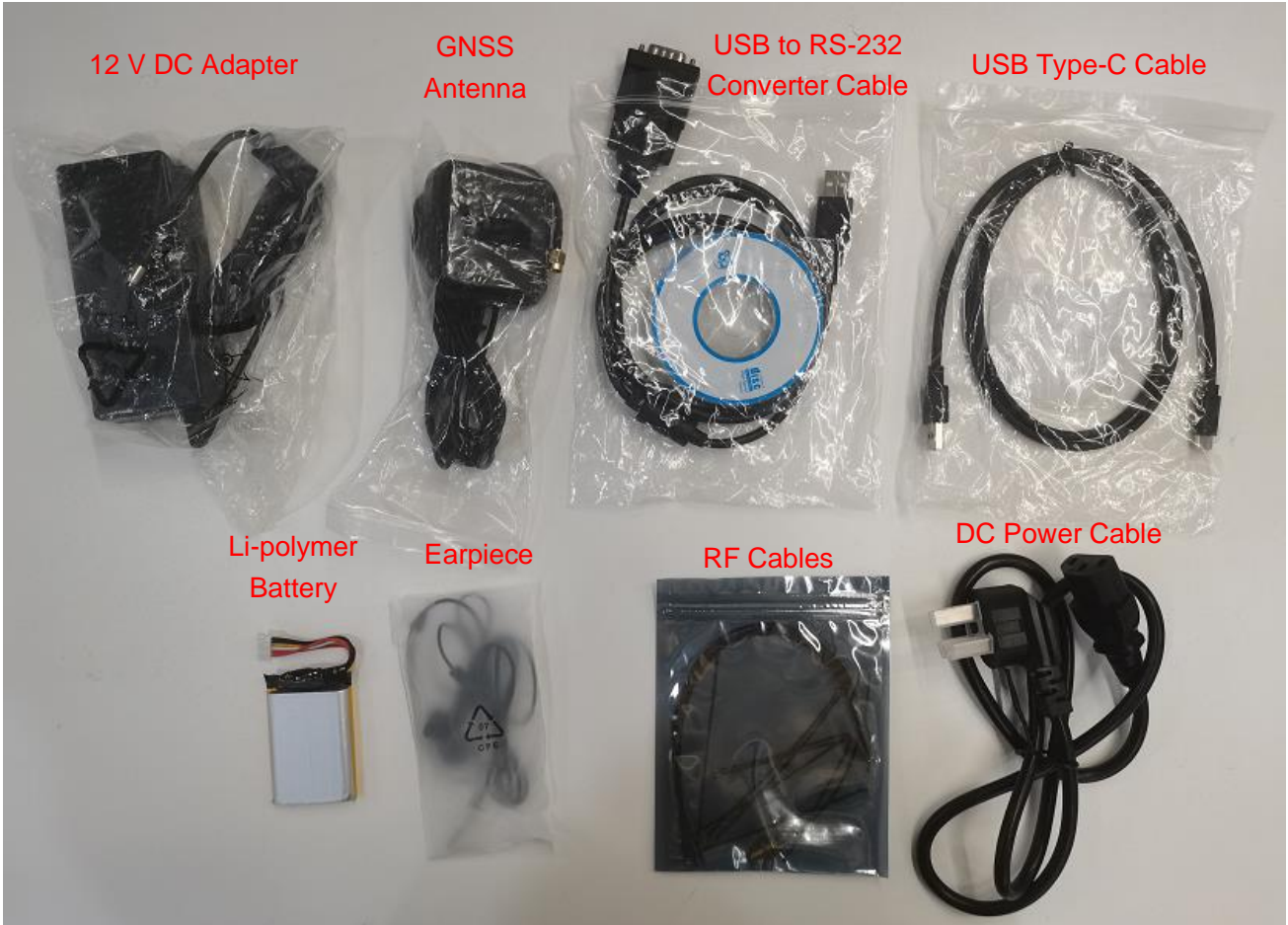
Figure 6: Smart 5G EVB Kit Accessories
