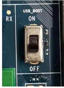
Figure 47: Emergency Download Switch
