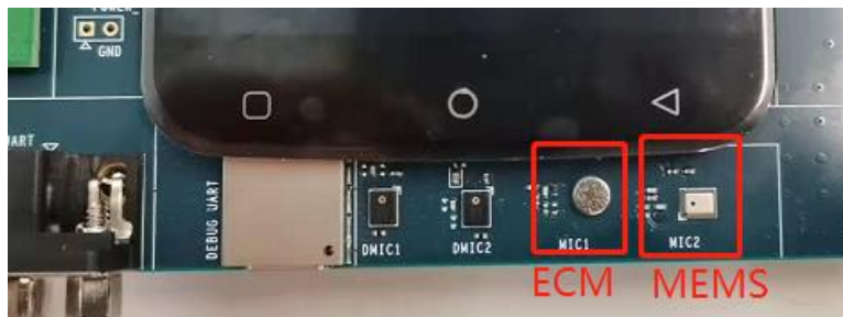
Figure 32: ECM-Type and MEMS-Type Microphones
