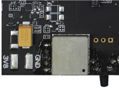
Figure 31: Debug UART Interface (J2005)
