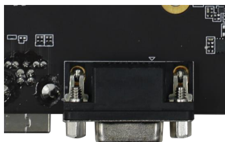
Figure 30: Main UART Interface (J2002)
