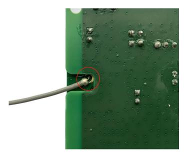
**Figure 16: Concentric Circle Welding**
