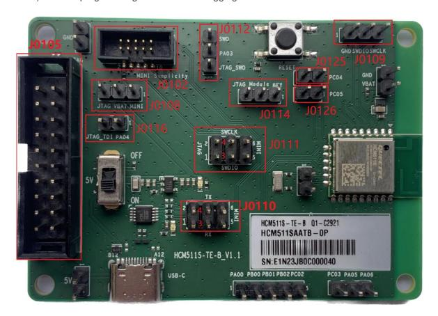
Figure 12: Debug and Jumper Interfaces
