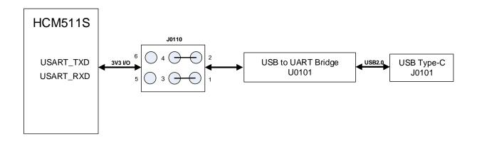
Figure 11: USB-to-UART Connection
