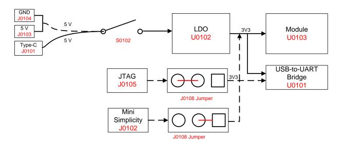
Figure 5: Power Supply for HCM511S-TE-B
