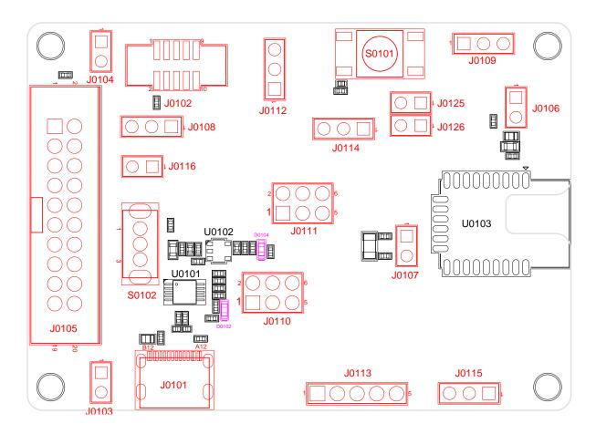
**Figure 3: Component Placement**
