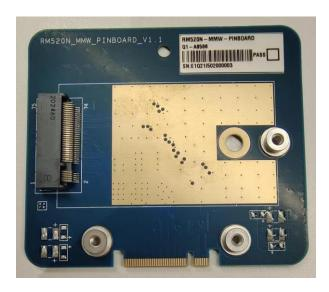
Figure 3: Top View of mmWave Pinboard
