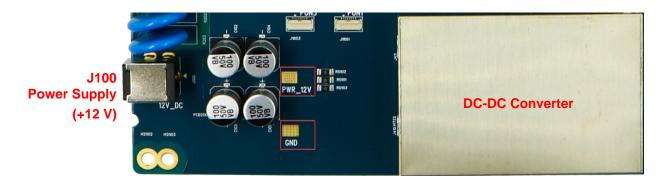
Figure 5: EVB Power Supply Interface
