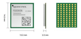
FGS060N is a high-performance Wi-Fi 6 and Bluetooth 5.2 module in LGA package launched by Quectel, complying with Thread protocol. Under the IEEE 802.11ax standard protocol, it supports MCS 0-MCS 11 rates in an 80 MHz bandwidth with 1024QAM supported. The module is designed with a reliable SDIO 3.0 interface to provide WLAN capability.
