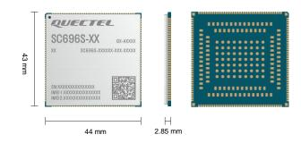
SC696S is a series of multi-mode Smart LTE Cat 4 modules with built-in Linux OS. Based on QCM6125 high-performance 64-bit octa-core processors with built-in Adreno<sup>TM</sup> 610 GPU, it is an ideal solution for a wide range of industrial and consumer applications requiring high data rates and multimedia functions. SC696S series comes in three variants: SC696S-EM, SC696S-NA and SC696S-WF (SC696S-WF only supports Wi-Fi and Bluetooth).
