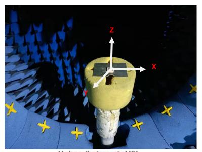
H plane: the tangent of XY E1 plane: the tangent of XZ E2 plane: the tangent of YZ
