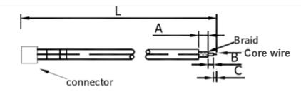
$\textbf{Connector}: \text{I-PEX MHF} \ , \ \text{Cable}: \text{RF Cable } \phi 0.81 \text{Gray}$
