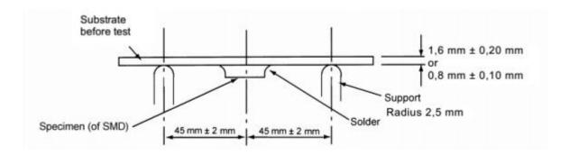
Weld the product to the central part of the PCB with the thickness 1.6  $\pm$ 0.2 mm or 0.8  $\pm$ 0.1 mm as the illustration shows, and keep exerting force arrow-ward on it at speed of 1 mm/s, and hold for 5  $\pm$ 1 seconds at the position of 1.5 mm bending distance, so far, any peeling-off of the product metal coating should not be detected.
