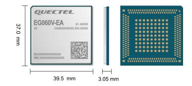
Quectel EG060V-EA is an LTE Advanced category 6 module optimized specially for M2M and IoT applications. Adopting the 3GPP Release 10 LTE technology, it reaches a maximum data rate of up to 300 Mbps downlink and 50 Mbps uplink.
