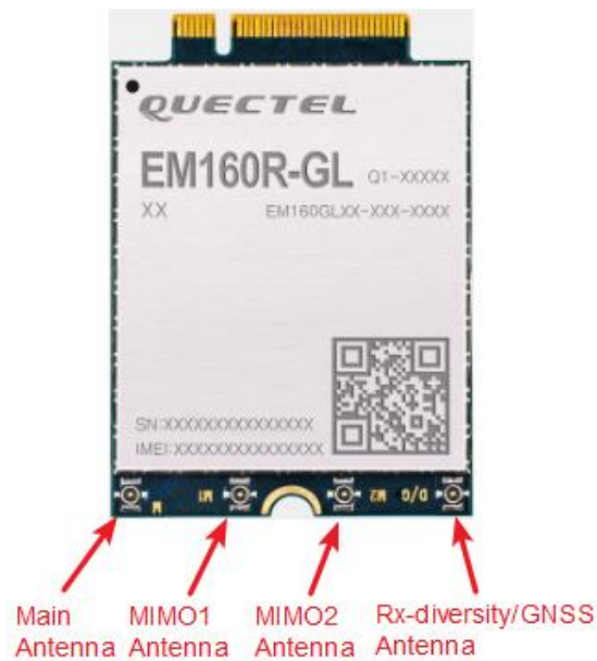
Figure 33: Antenna Connectors on the EM160R-GL Module
