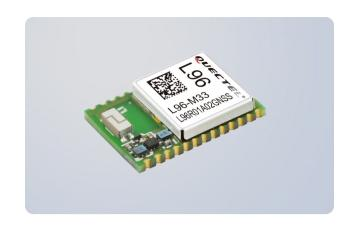
L96 is a concurrent multi-GNSS receiver module with embedded chip antenna. With 33 tracking channels, 99 acquisition channels and 210 PRN channels, L96 supports concurrent reception of up to three GNSS systems (GPS+GLONASS+Galileo). The built-in LNA provides the module with better performance under weak signal areas. The embedded chip antenna reduces the total size of customers' applications. To meet varied application demands, L96 also provides an external antenna interface.
