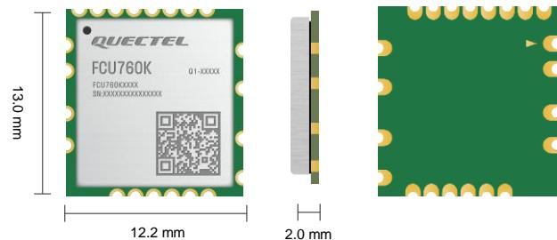
FCU760K is a high-performance Wi-Fi 6 and Bluetooth 5.4 LCC package module launched by Quectel, which can be used for WLAN and Bluetooth connections. The module complies with IEEE 802.11a/b/g/n/ac/ax protocol, supports up to 11ax MCS 11 rate at 80 MHz channel, and the transmission rate can reach 600.5 Mbps. FCU760K adopts reliable USB 2.0 interface design and supports WLAN/Bluetooth high speed transmission.
