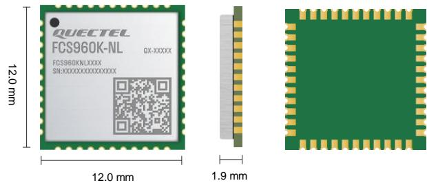
FCS960K-NL is a high-performance Wi-Fi 6 and BLE 5.4 module launched by Quectel, which can be used for WLAN and BLE connections. The module complies with IEEE 802.11a/b/g/n/ac/ax protocol and supports a bandwidth of up to 40 MHz, with a maximum transmission rate of 286.8 Mbps, and features a reliable SDIO 3.0 interface design, enabling high-speed WLAN transmission.
