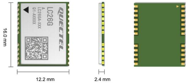
LC26G (AB) is a multi-constellation GNSS receiver module capable of tracking GPS, GLONASS, Galileo, BDS and QZSS concurrently. LC26G (AB) is designed to be compatible with Quectel L26 and L26-LB modules, allowing for smooth migration between them.
