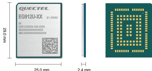
Quectel EG912U is a series of the LTE Cat 1 module optimized specially for M2M and IoT applications. It delivers maximum data rates up to 10 Mbps downlink and 5 Mbps uplink. Designed in the compact and unified form factor, EG912U series is compatible with Quectel multi-mode BG95 series, BG96, EG91 series, EG95 series and EG915U series modules, ensuring that it can easily migrate between 2G and 4G network to meet the needs of different industry applications.
