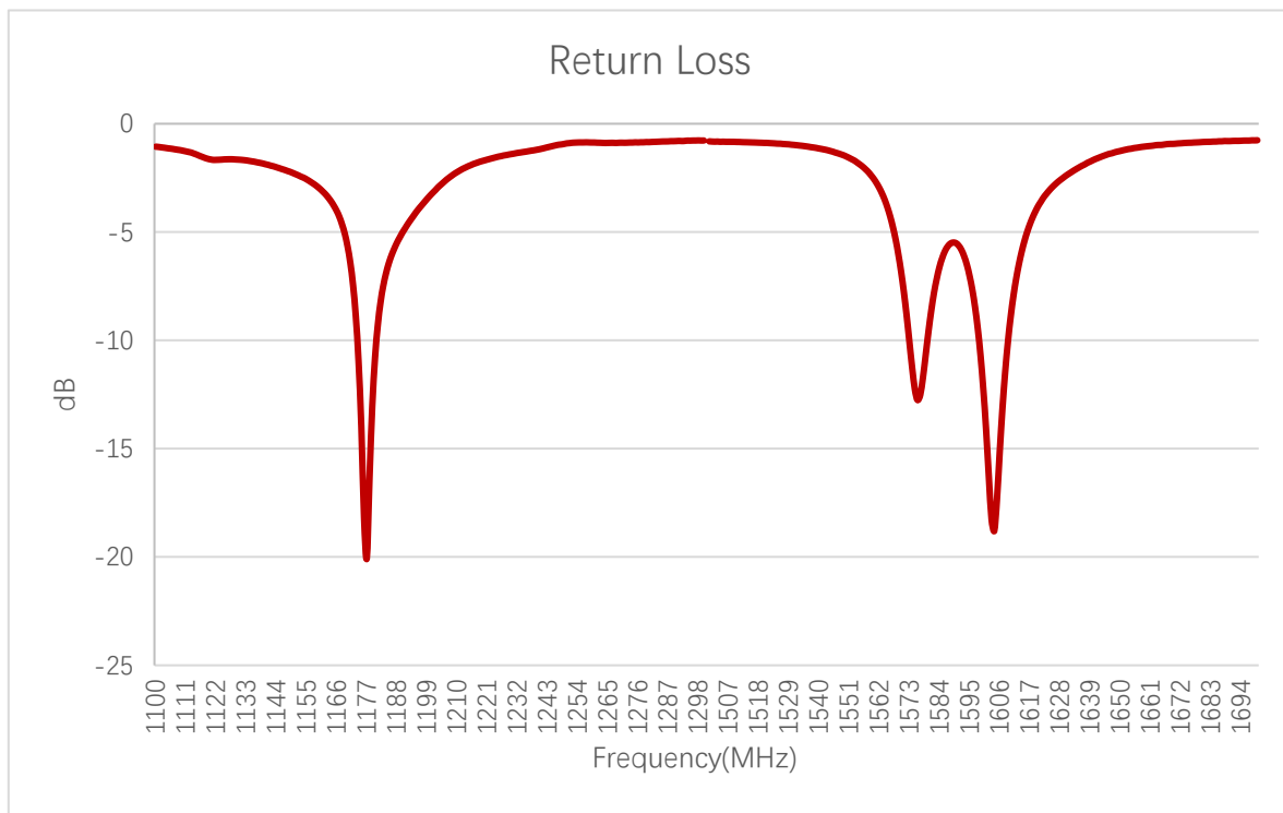
Return Loss (dB) – GNSS
