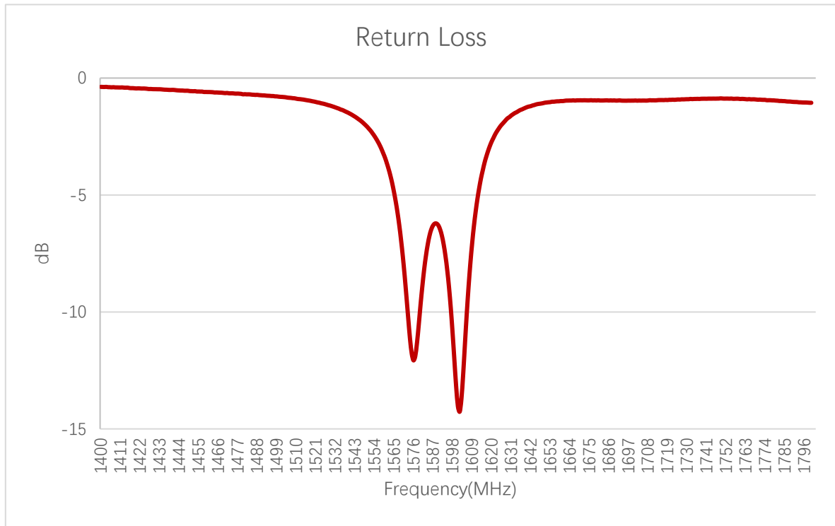
Return Loss (dB) – GNSS
